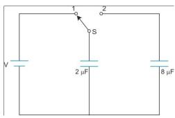
A capacitor of 2  $\mu F$  is charged as shown in the diagram. When the switch S is turn to position 2, the percentage of its stored energy dissipated is:
